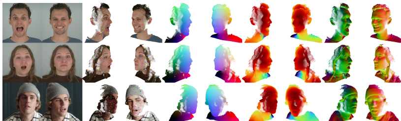
Fig. 1: Face Anything. Unified 4D facial reconstruction and dense tracking from image sequences via joint prediction of depth and canonical facial coordinates. Left to right: RGB input, 4D reconstruction with tracks, canonical maps, depth maps, and normal maps. Website: https://kocasariumut.github.io/FaceAnything/
